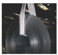
We are manufacturer of round endless slings by using HMPE yarn in higher capacity upto 500 Ton round endless slings, manufactured by using HMPE yarn in higher capacities up to 500 Ton. These slings have top most degree of perfection. These are suitable to specialized extreme heavy lifting requirements. These slings are available in Round Endless, Eye and Eye type and TWO PATH Sling type.
