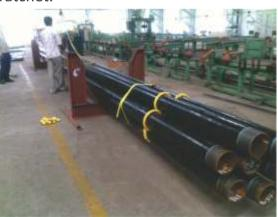
For coated pipe, buckles will also be coated so that no scratches will be on pipes. Process of lashing is illustrated as below
