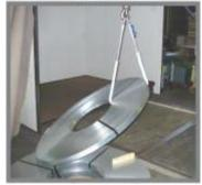
The description of Dynaflexx sleeves need to come under - Another Innovation is Dynaflexx. Cut resistant Kevlar/HMPE sheet stitched with Velcro. Most efficient in low temperatures and can lift products with protruding sharp points, weld spats. This sleeve provides cushion and protection both. The sleeve allows sling to slide in freely providing maximum wear resistance.
