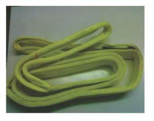
100% High Tenacity Polyester. Made of 3 & 4 thickness of Webbing. Flat & Wide Load Bearing surface. According to EN 1492-1:2000 or ASME B 30.9. Safety Factor 7:1 and 5:1. Low Stretch Factor: Elongation 3-7%. High strength to weight ratio: Weight 80% less than Equivalent Wire or Chain Slings. Available upto 300 mm width & 24 Ton Capacity. Colour coded for easy identification. Maximum working temperature 90°c. Anti-abrasion sleeves and anti-cutting sleeves protection (optional).
