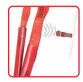
ALL FERRRETERRO PREMIUM<sup>®</sup> Sling comes with strategically placed microchip inside layers of slings which is water and chemical resistant. The chip contains a Unique no. in digits which gives the no. and details of sling, manufacturing date, dispatch details and vital information of the sling. The transponder works within 10"range and is a great boon for safety and auditing purpose.
