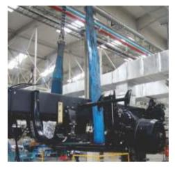
Now all your turning devices for turning automobiles, chassis, Marble Blocks, Machines, Moulds infact, rather anything can be secured on our range of Ferreterro ROTOMAXX slings. These are heavy duty slings impregnated with Polyurethane and plasticized coating to grip the load and are almost Anti-cut. These silngs can be made up to 30 ton load turning.
