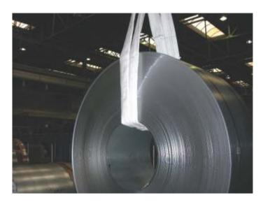
For Many applications we need Synthetic slings where the temperature of the product goes upto 180 degrees or more. We manufacture slings with triplet heat resistance, load bearing sleeves which hug the product and bear most of the heat. The sleeves are designed so as to minimize the heat transfer to the inner core sling. These slings work safely till 160 degrees of temperature and to be used with strict guidelines laid by Ferreterro.
